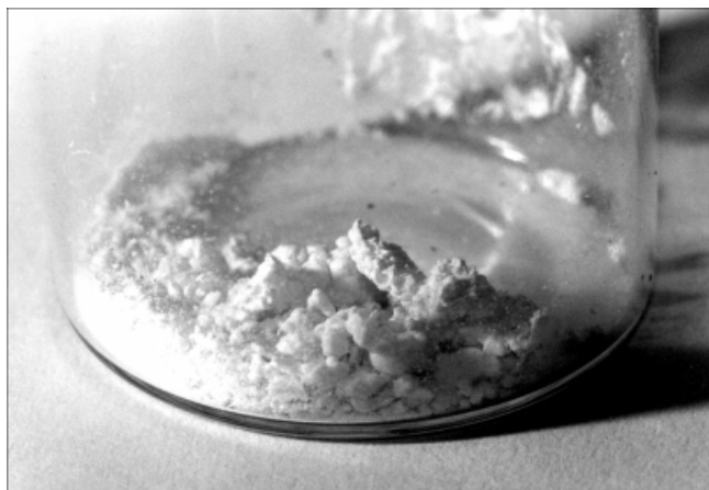
Photo 2. Yellow product obtained during the oxidation of NaK alloy by argon and air sweeping (Table 7, test 1)
