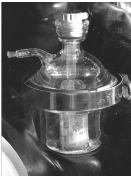
Photo 4. Product obtained during the oxidation of NaK alloy by argon and air bubbling for three months (Table 8)
