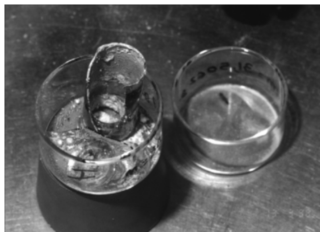
Photo 1. Results of the reaction between NaK alloy and sodium peroxide hydrated in air (Table 6, test 3b)
